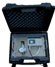
Compressed air quality measurement
