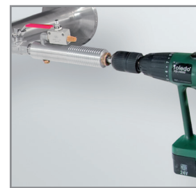
Drill under pressure with the CS drilling jig
